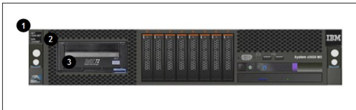
Figure 6. The DDS Generation 5 USB Tape Drive installed internally in an x3650 M3 server
