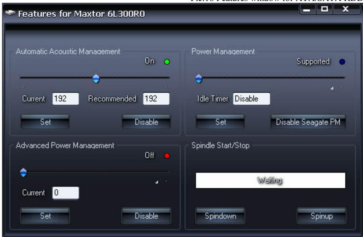
The program can show defect-lists and start or stop spindle for SCSI drives.
