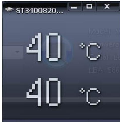
For SCSI drives the information window shows two values. The second value is shown on the Task bar and represents current temperature. The first value indicates maximum allowed temperature for HDD.
