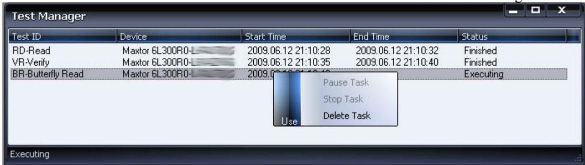
This window contains test queue. All surface tests, S.M.A.R.T. tests and Temperature Monitor tests will be displayed in the Test Manager. Manager allows deleting tests from queue; some test could be paused or stopped.
