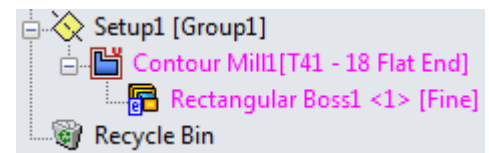
Generated Operation listed in Operation Tree
