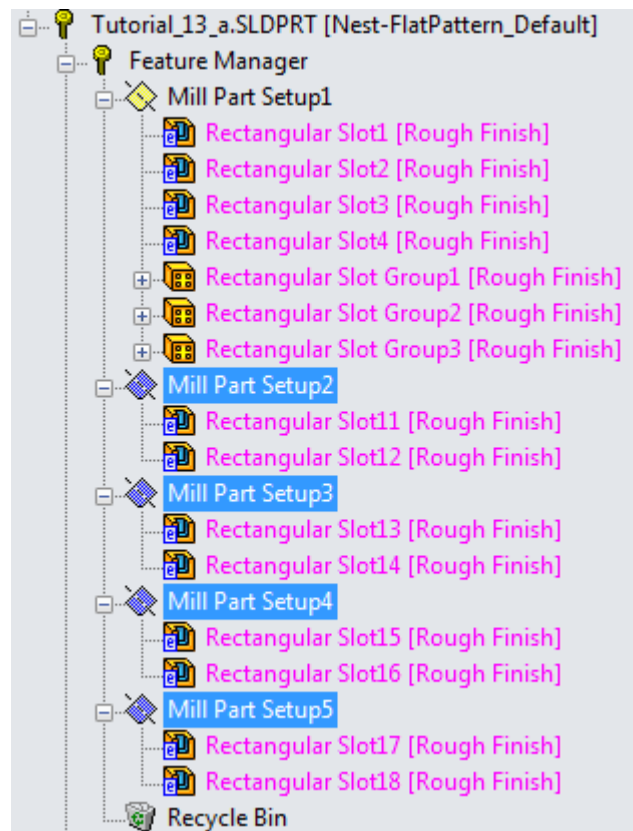
Selecting the Mill Part Setups to delete it
