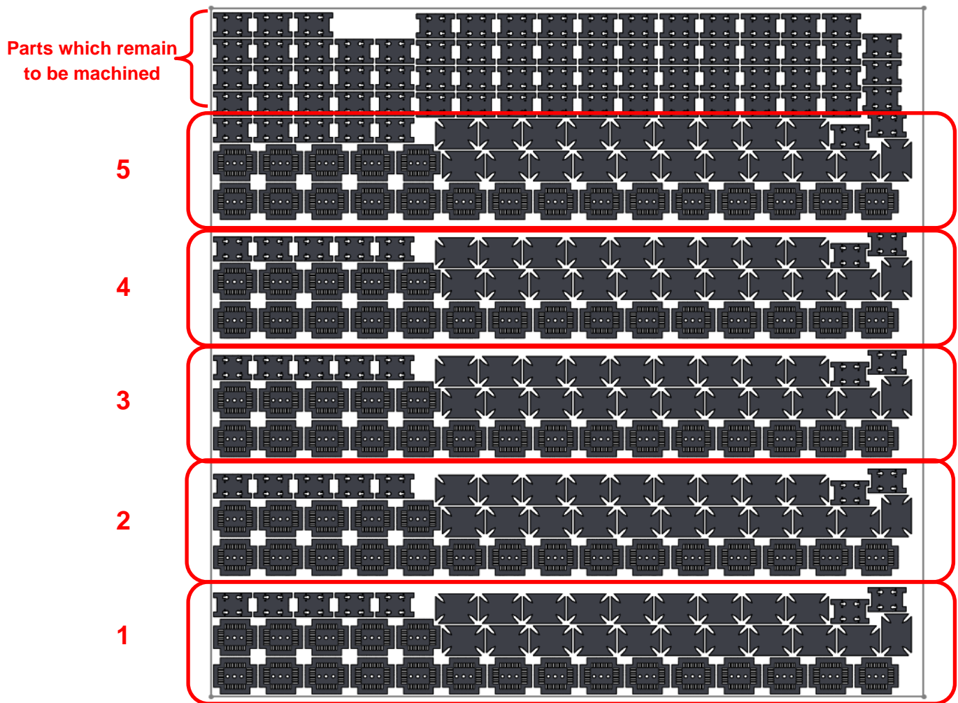
Nesting layout with 5 identical regions created using 5 tool heads
