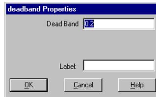
**Dead Band:** Indicates the width of the zone of lost motion about the input signal's 0 value. The default is 0.2.
