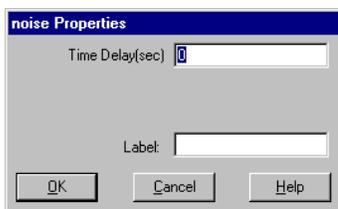
**Time Delay(sec):** Indicates, in seconds, how long to delay before calculating the value of the noise signal. The default is 0.
