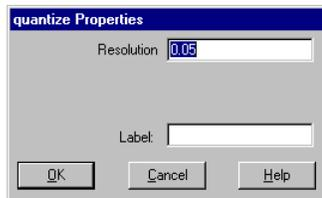
**Resolution:** Specifies the value to which the input signal is rounded or truncated. The default is 0.05.
