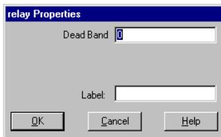
**Dead Band:** Indicates the width of the zone of lost motion about the input signal's 0 value, thereby creating a tri-state relay operator (-1, 0, 1). When input is less than half the negative Dead Band value, the `relay` block outputs -1. When input is greater than half the positive Dead Band value, the `relay` block outputs +1. When input lies within the range (-Dead Band/2, +Dead Band/2), the `relay` block outputs 0. You cannot specify a negative value for this parameter. The default is 0.
