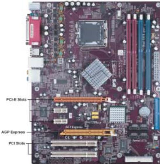
**PCI-E1 Slots** The PCI Express x16 slot is used to install an external PCI Express graphics card that is fully compliant to the PCI Express Base Specification revision 1.0a.
