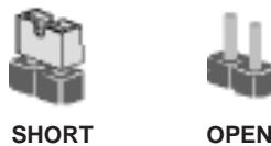
This illustration shows a 3-pin jumper. Pins 1 and 2 are SHORT
