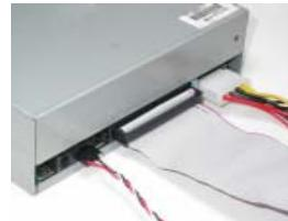
IDE devices enclose jumpers or switches used to set the IDE device as MASTER or SLAVE. Refer to the IDE device user's manual. Installing two IDE devices on one cable, ensure that one device is set to MASTER and the other device is set to SLAVE. The documentation of your IDE device explains how to do this.
